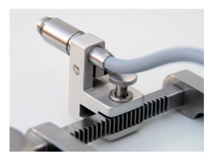
This anodized aluminum fixture mounts on the rack of the Buxton Shoulder retractor and accommodates a flexible, fiber optic rod to illuminate the wound site. The attachment has a clamp opening of 8 mm and can be mounted on most any device with parallel surfaces.
